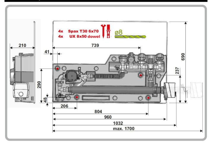
The ASKOWALL-OP can be attached to the wall using the four screws supplied.
