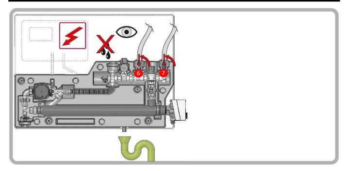
After opening the two shutoff of flow and return (no. 6 & 7), the system must be checked for leaks. No water leakage may be detected.
