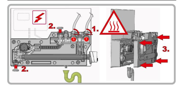
**ATTENTION:** Before closing the insulation cover, the two shut-off valves of flow and return (no. 6 and no. 7) must be closed. Otherwise the insulation cover cannot be closed.
