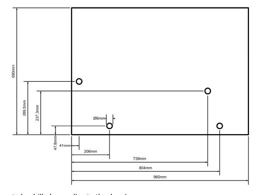
The holes have to be drilled according to the drawing.
