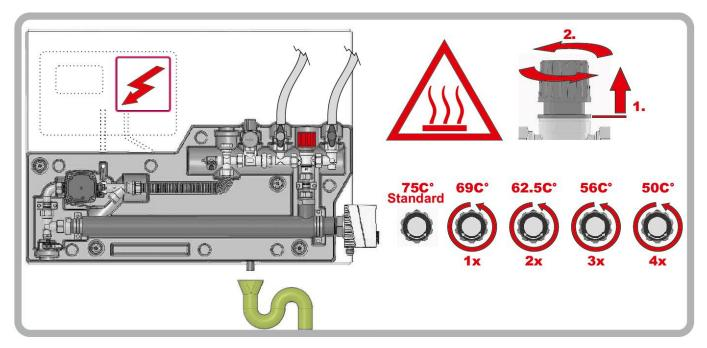
Setting the output temperature to the buffer tank (opening temperature of the thermostatic valve)
